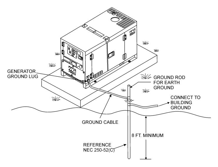
Figure 12. Typical Generator Grounding Application
